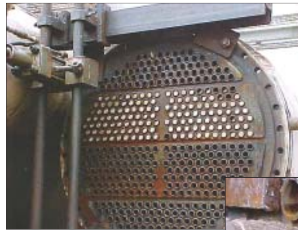
At left, a heat exchanger loaded with Hydrokinetics bullet plugs. Below, a Hydrokinetics nozzle about to enter a tube. Bottom photo, pieces of scale removed from tubes.
