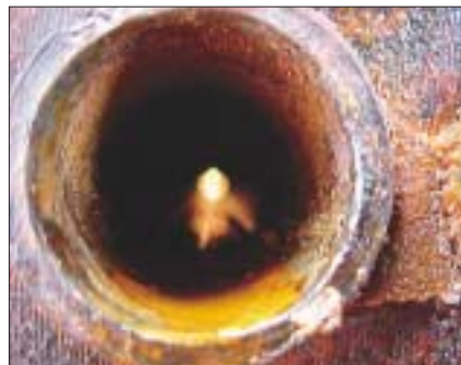
Upper photo, heat exchanger tubes before Hydrokinetic cleaning; lower photo, entry to tubes after Hydrokinetic cleaning.
