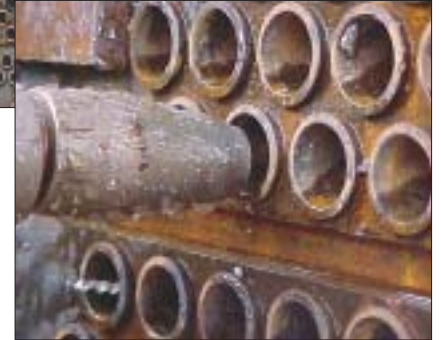
At left, a heat exchanger loaded with Hydrokinetics bullet plugs. Below, a Hydrokinetics nozzle about to enter a tube. Bottom photo, pieces of scale removed from tubes.
