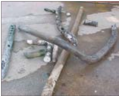
Top photo, foulant exits a pipe during Hydrokinetics cleaning. Bottom photo, foulant comes out in a snakelike fashion.
